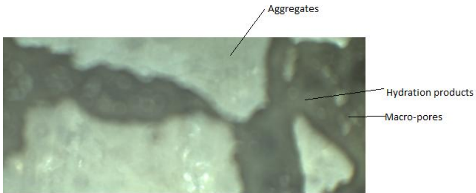
Figure 12: x200 magnification - sample three
