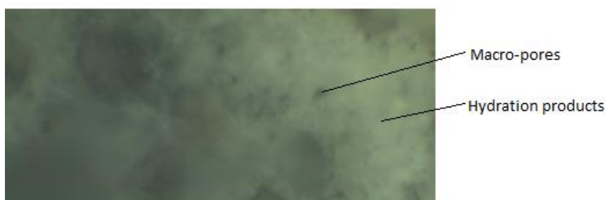
Figure 11: \times 1000 magnification - sample two
